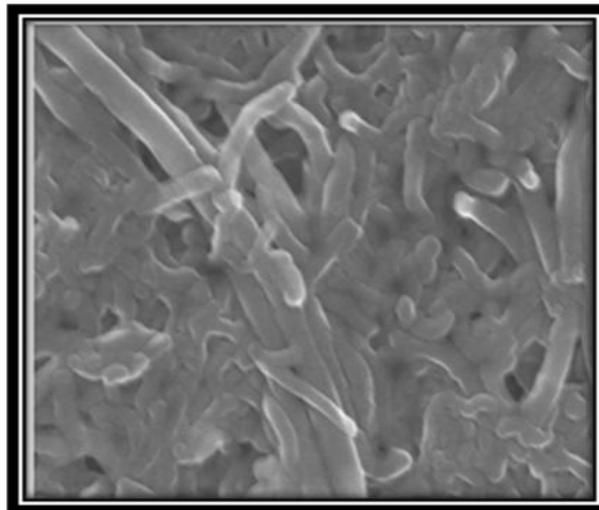
Fig 3: Scanning electron microscopy of Functionalized MWCNT.
