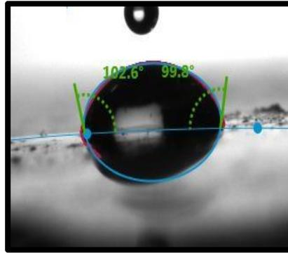
Fig 9: Contact angle measurement of 0.5% MWCNT in Epoxy resin (EC-5).
