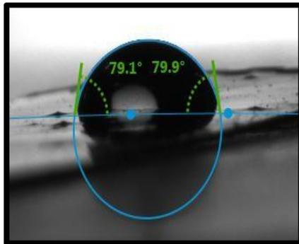
Fig 7: Contact angle measurement of 0.1% MWCNT in Epoxy resin(EC-1).
