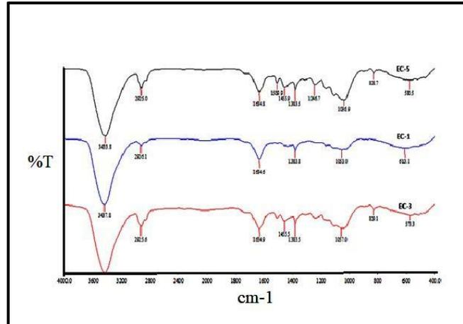
Fig 2 : FTIR spectra of MWCNT/epoxy nanocomposites (EC-1, EC-3 and EC-5)
