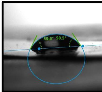
Fig 10: Contact angle measurement of pure Epoxy resin (EC).
