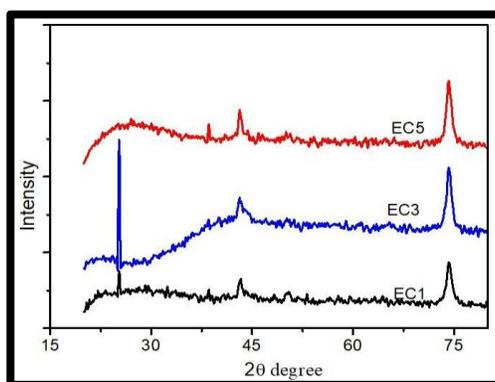
Fig 1: X-ray diffraction of EC-1, EC-3 and EC-5.
