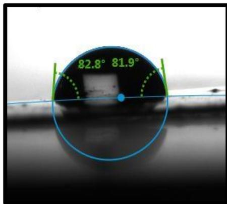
Fig 8: Contact angle measurement of 0.3% MWCNT in Epoxy resin(EC-3).
