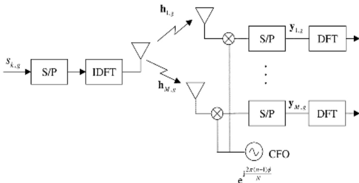
Fig.1. Illustration of OFDM system with multi-antenna receiver
