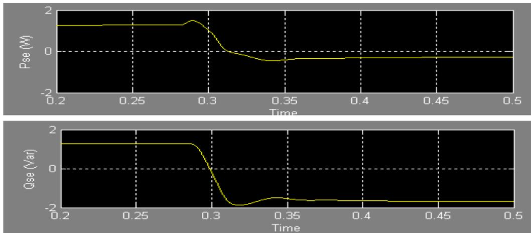
Figure. 10 Step response of the DPFC: active and reactive power injected by the series converter at the fundamental frequency
