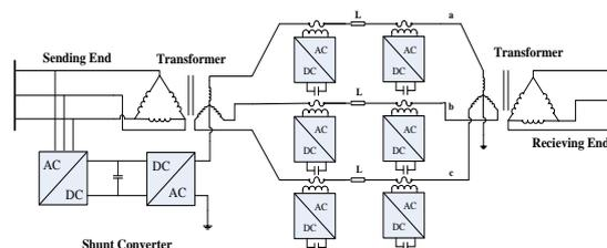
Figure. 3 DPFC Connections in Three Phase
