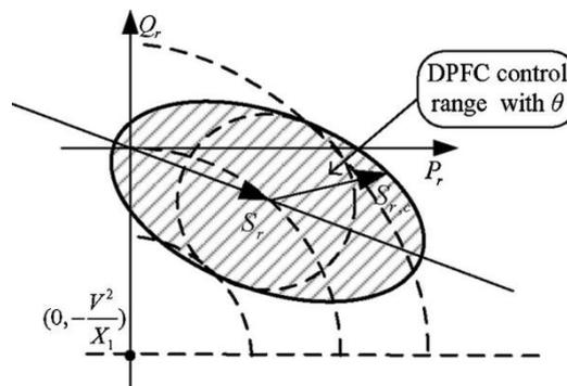
Figure .5 DPFC power-flow control range.
