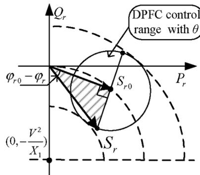
Figure. 4. Maximum Active Power Requirement of Series Converter
