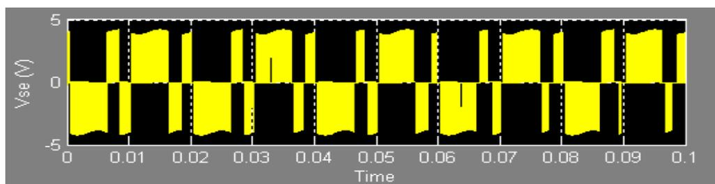
Figure. 7 DPFC operation in steady-state: series converter voltage
