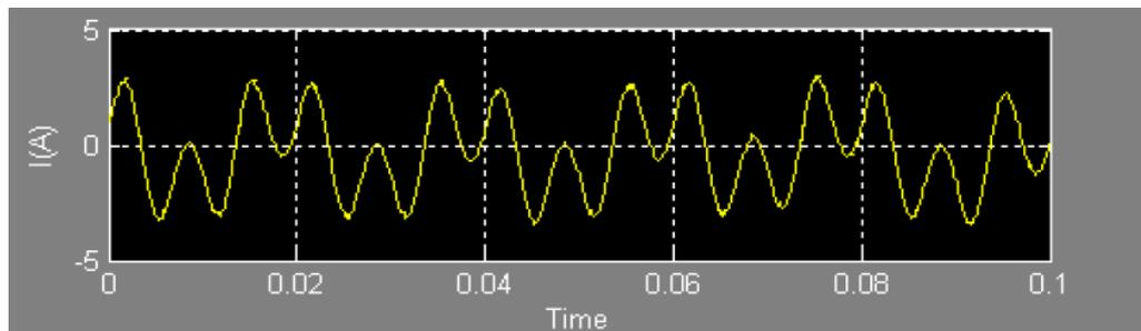
Figure. 6 DPFC operation in steady-state: line current
