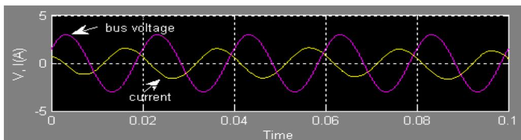
Figure. 8 DPFC operation in steady-state: bus voltage and current at the  $\Delta$  side of the transformer
