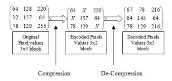
Figure 5: Modified TiBS encoding-decoding Process
