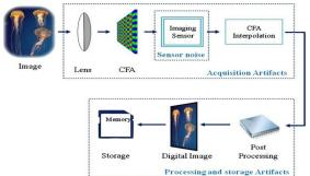
Fig1: A schematic view of a standard digital image acquisition pipeline.
