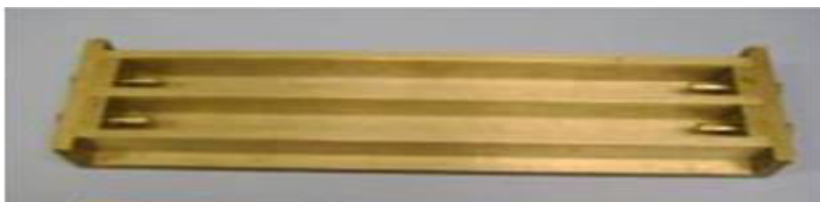
Figure 3.1 Drying Shrinkage Mould Specimen (Source: Google)
