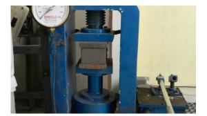
The test was carried out conforming to IS 516-1959 to obtain Split Tensile Strength of Concrete strength at the age of 3 days ,7 days and 28 days.
