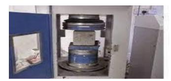
Compressive Strength of Concrete Test, Result & Calculations
