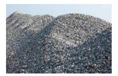
Coarse aggregate of size 20 mm of crushed stone locally available confirming to IS 383-1987 was used
