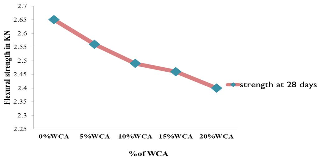
**Fig. 2:** Represents the variation of flexural strength with percentage replacement of WCA for M25 grade concrete
