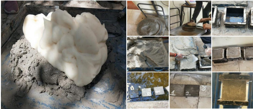
Image: Foam concrete mixing
