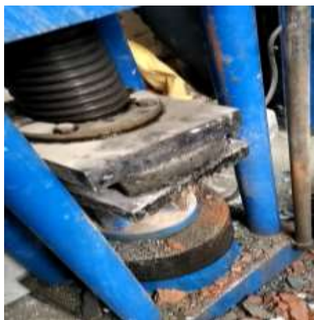
Fig :- Compression testing on paver block
