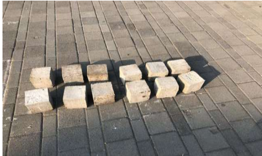
Fig: Sun Drying of Blocks
