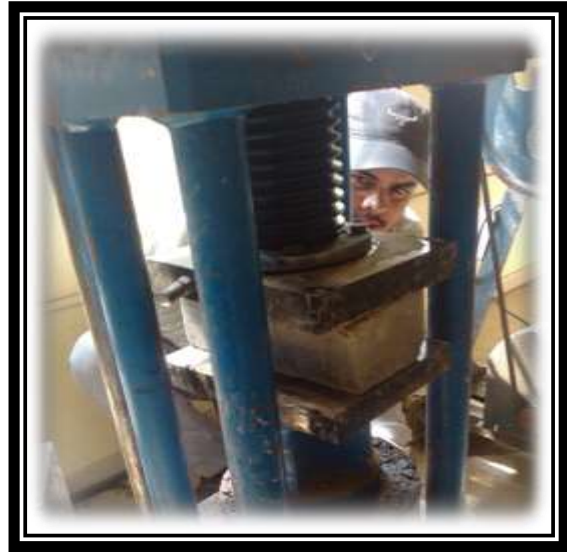
Fig. 13 Testing of Bricks
