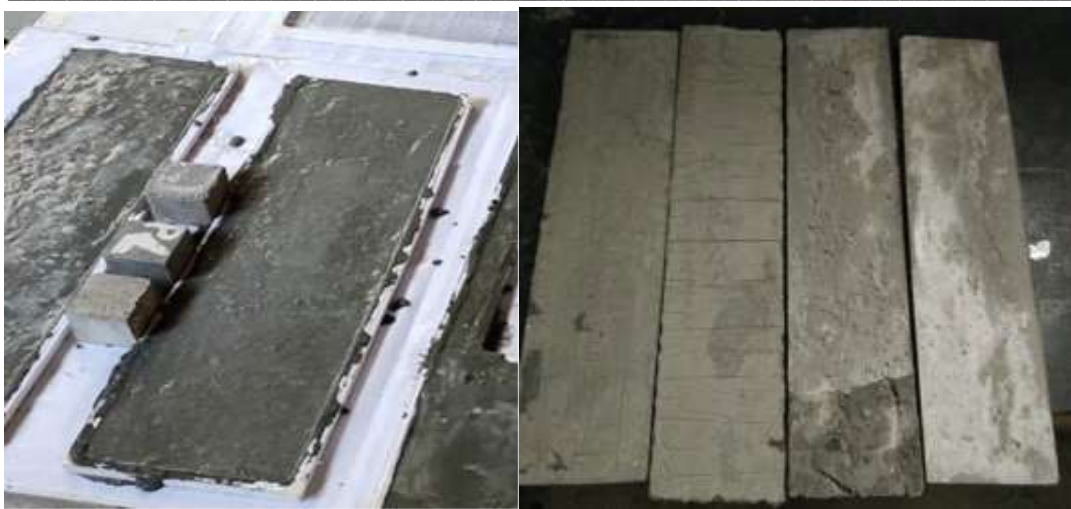
Fig. casting of AAC panels
