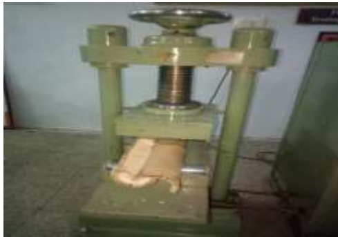
Fig 5- Flexural strength test on sample 1
