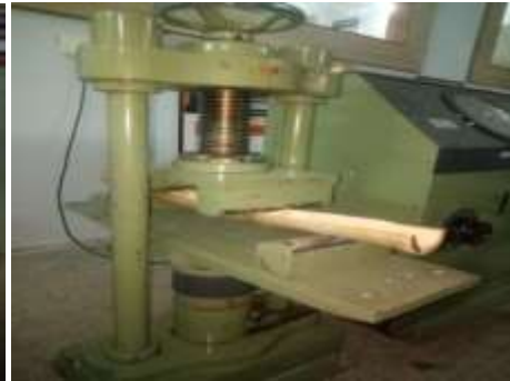
Fig6. Flexural strength test on sample 2
